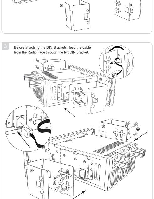
Using the 8 screws included in the Radio Motor box, install the DIN Brackets (included with the DIN Kit) to the sides of the Radio Motor. Adjust the brackets forward until they meet the back of the radio face. Be careful not to bend the brackets to ensure proper fitment into the DIN Sleeve. Plug the cable from the Radio Face into the Radio Motor.
